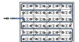
A centralized piping system permanently fixed on the battery cells, delivers to them low pressure air (requires an airlift configured charger). This air is mixing the electrolyte solution with many and significant benefits for the battery life and its related costs:
